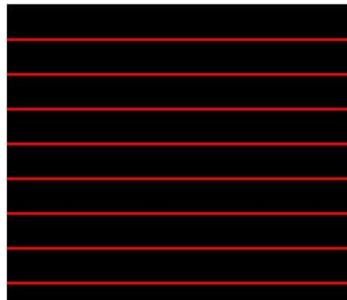
Figure 2.2. LCD is filled with horizontal lines.
